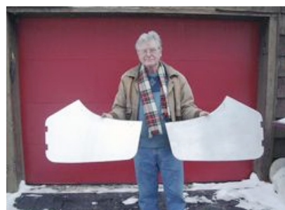
Ron Lindemann, reskined the doors in aluminum
