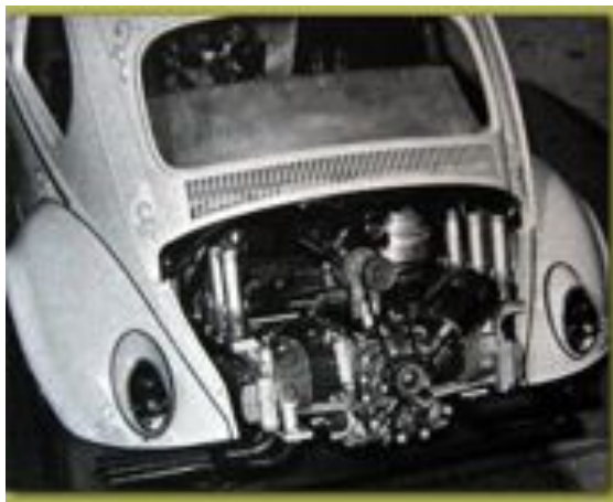
VW Beetle with a Corvair Engine
