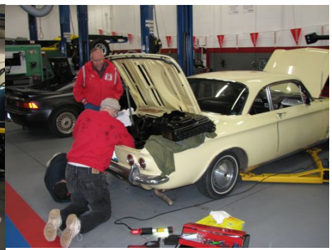
Bill Boudway gets our Chief Tech., Dave Ellis to help replace the rear main seal on Grace's car. Jim B. Acted as Tech and advisor.
