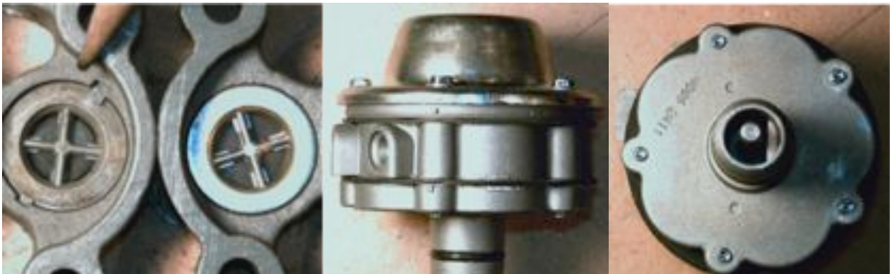
Valves on current pump (left) are fully seated and staked. Improved diaphragm material. Lot number stamped on bottom.
