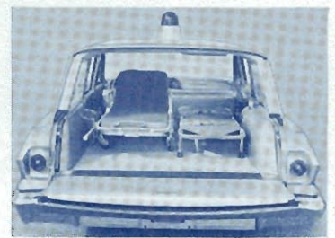
There's plenty of width to handle second patient on wheeled emergency stretcher which is standard equipment in 1963 Amblewagons. Even two full length 19" cots fit satisfactorily.
