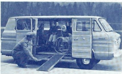
A-661 Self-Storing Entrance Ramp covered with non-skid material and auxiliary floor.
