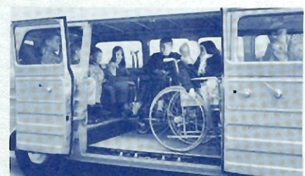
A-662 Wheel-Chair Tie-Downs to hold three chairs securely in position.
