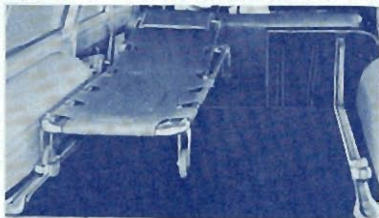
A-217 Telescoping Cot locked into track in extended position. Split second seat raised for attendant.
