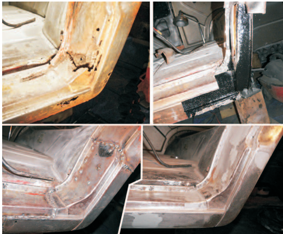
Front door dog-leg repair. Typical of several other areas, rotted metal was replaced with salvage parts when available.
