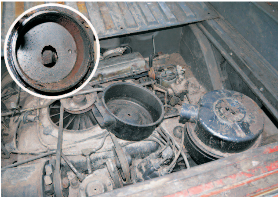
Engine as found in 2016. Inset shows one of the pistons with a detonation hole.
