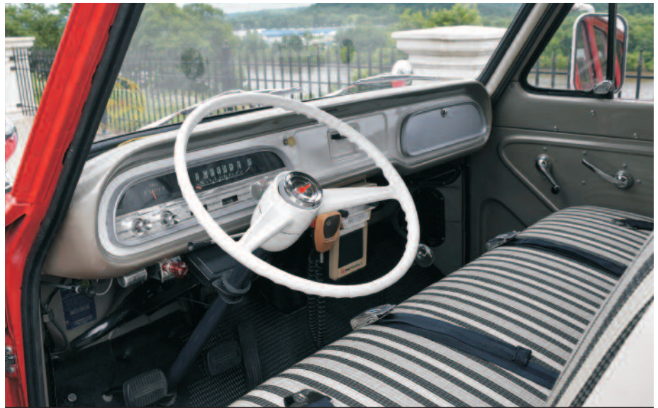
Restored cab. Notice Motorola Motrac radio head located in place of standard radio.
