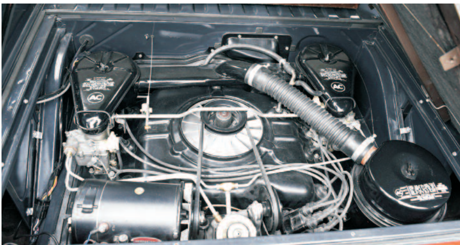
Engine restored with LCI generator and pre-oil bath air cleaner.
