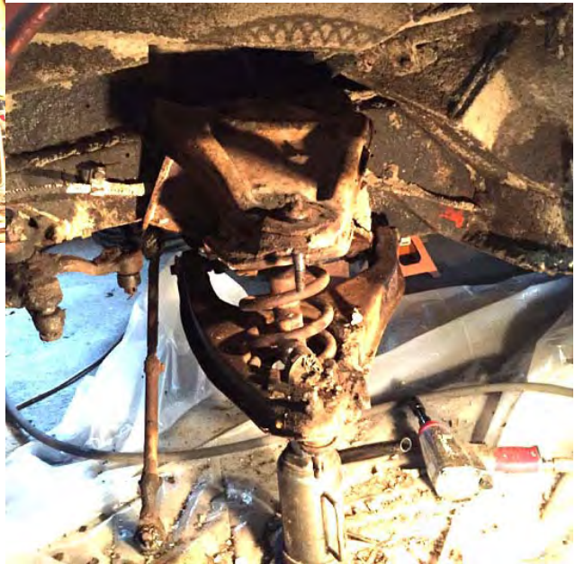
Front suspension under way. Like everything else, covered with undercoating and caked with rock-hard mud; literally had to chisel some off. Spring extraction went well; had to cut off shocks at bottom.
