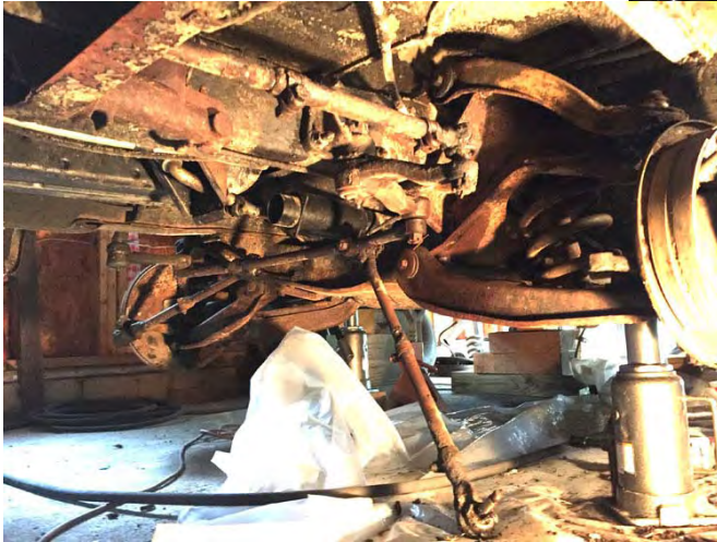
Front suspension under way. Like everything else, covered with undercoating and caked with rock-hard mud; literally had to chisel some off. Spring extraction went well; had to cut off shocks at bottom.
