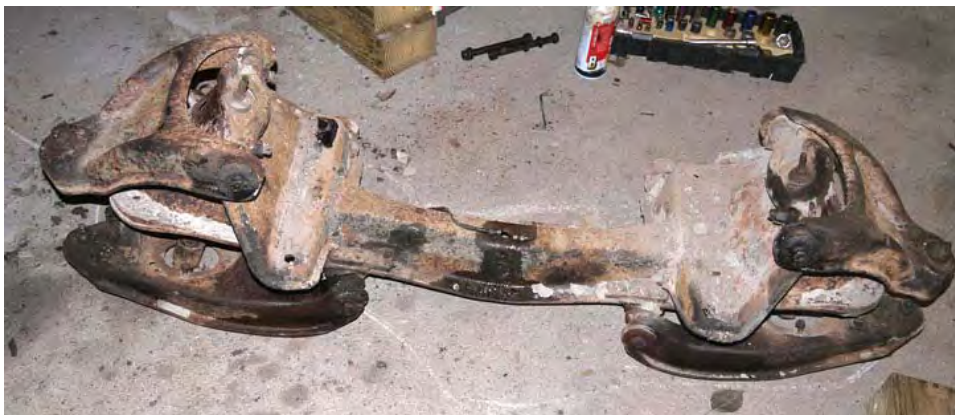
Front crossmember removed. The bolts holding to the undercarriage were extremely difficult to remove, but they succumbed without incident.
