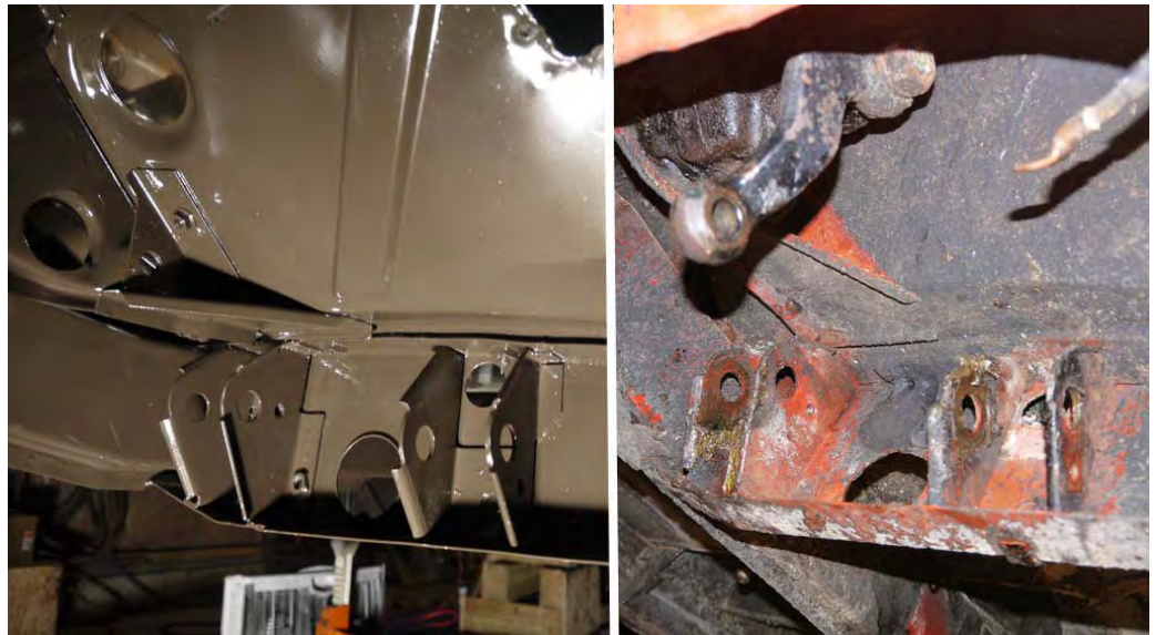
pedal bushing brackets after / before:
