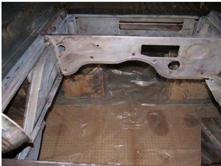
Any areas with surface rust have been spot painted with POR-15. Darn good stuff, but needs to be lightly sanded before applying paint. Of course the silver lining of an abundance of undercoating is that there is not much rust. However, I will need to come back later to repair some damaged areas.
