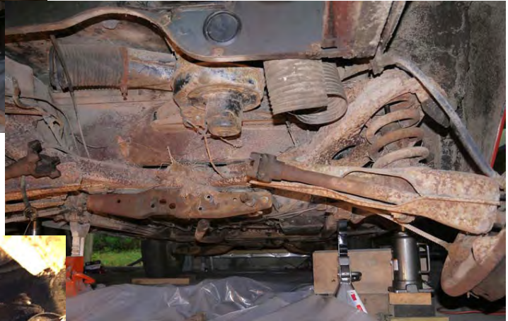
Rear suspension ready for removal. Brake flanges and axle yokes came off without too much trouble, as did the bolts holding the rear crossmember to the undercarriage.
