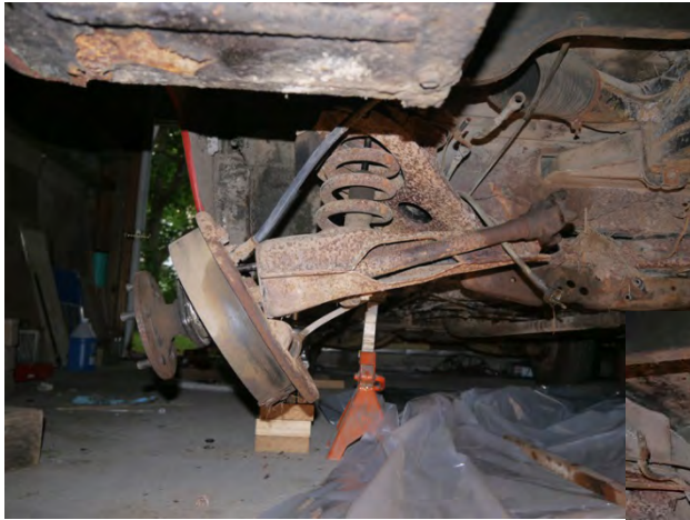
Rear suspension ready for removal. Brake flanges and axle yokes came off without too much trouble, as did the bolts holding the rear crossmember to the undercarriage.
