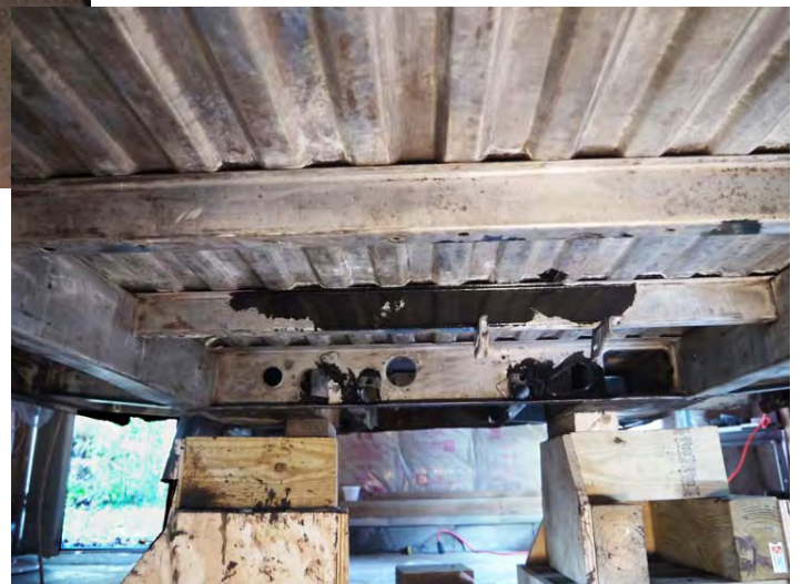
Any areas with surface rust have been spot painted with POR-15. Darn good stuff, but needs to be lightly sanded before applying paint. Of course the silver lining of an abundance of undercoating is that there is not much rust. However, I will need to come back later to repair some damaged areas.
