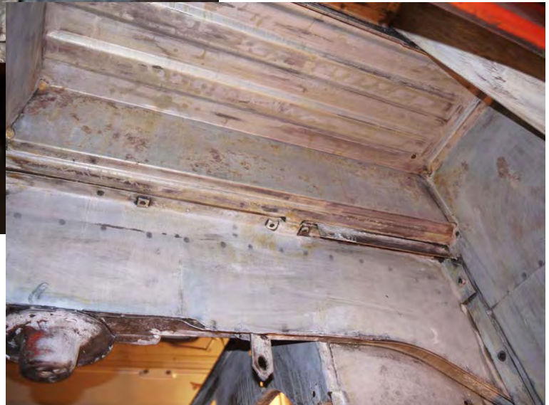
Any areas with surface rust have been spot painted with POR-15. Darn good stuff, but needs to be lightly sanded before applying paint. Of course the silver lining of an abundance of undercoating is that there is not much rust. However, I will need to come back later to repair some damaged areas.
