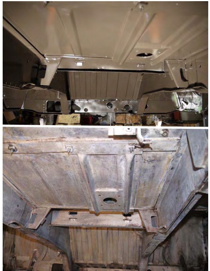
It took a lot of work to clean all the crevices, such as around the gas filler opening
