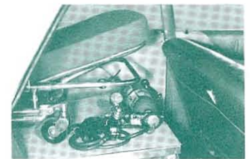
A-501 Portable Oxygen Inhalator mounted near attendant's seat.
