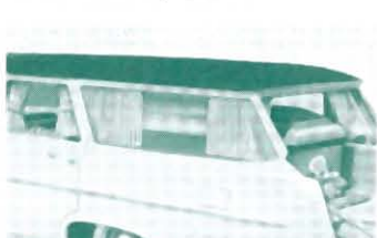
A-401, 402, and 403 Drapes are mounted on removable chrome frames.
