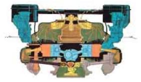
FORCED-AIR COOLING controls engine temperature efficiently and directly, without the intermediate stage of a liquid coolant which must be air-cooled in a radiator. A high-capacity blower blasts cooling air between cylinder barrels and through passages in the heads, where it picks up heat directly from deep, efficient cooling fins. A thermostatically controlled ring damper governs the air supply to the blower, speeding engine warmup and stabilizing operating temperature automatically.
