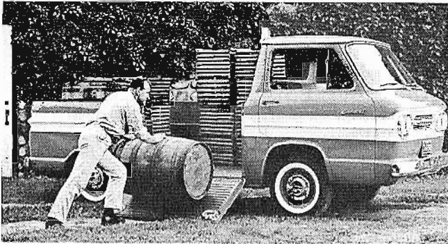
THE EXCLUSIVE CARGO RAMP on the Corvair 95 Rampside model permits loading of heavy objects without lifting. When closed, the ramp fits securely into the body side.
