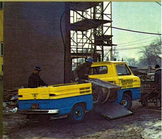
Corvair 95 pickups are available in both Loadside and Rampside models. The Rampside offers the extra convenience of direct, curb-level access to the central cargo floor. In either model, Corvair 95 design is a natural for camper body installation, with the drop-floor section making possible full stand-up headroom inside with minimum overall outside height. Rampside camper units offer walk-in, side-door convenience.
