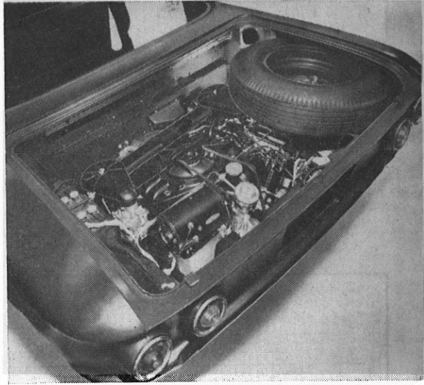
Flatter, separate air cleaners at each carb lower Corvair engine enough to make room for tire in the rear. This in turn increases the available luggage space, up front, as shown above.
