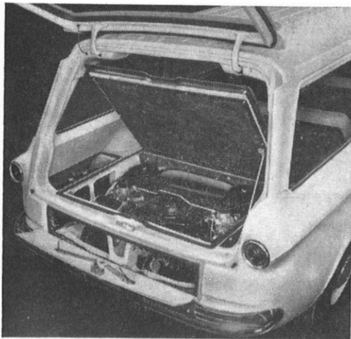
With Corvair's engine air cleaner superstructure gone, engine fits into new Lakewood wagon.
