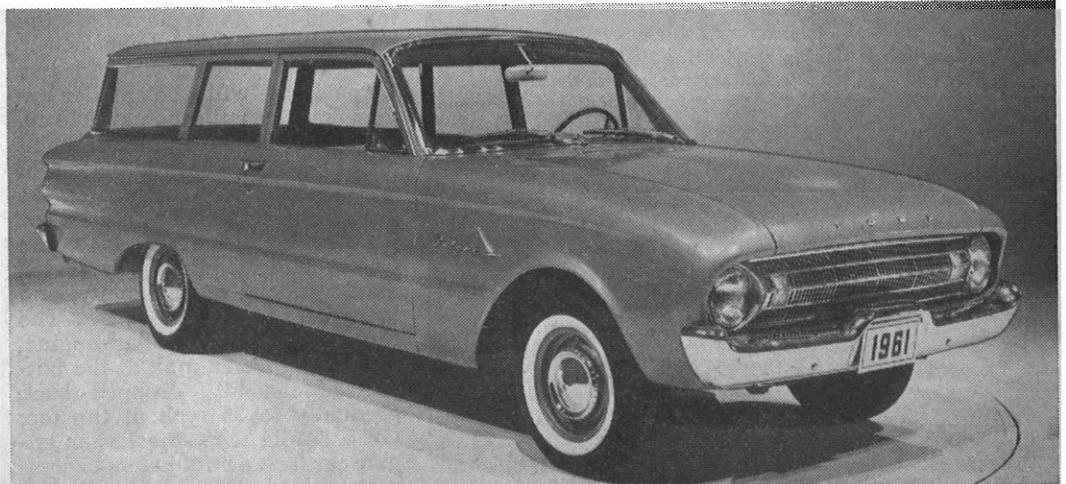
Falcon for '61 gets a new grille and a 101-hp engine option with longer stroke for better torque.
