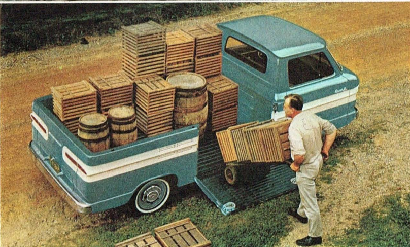
CORVAER 95 RAMPSIDE—The only pickup with a built-in side loading ramp!
