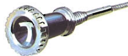
MANUAL THROTTLE CONTROL Permits driver to manually adjust throttle to any engine speed.
