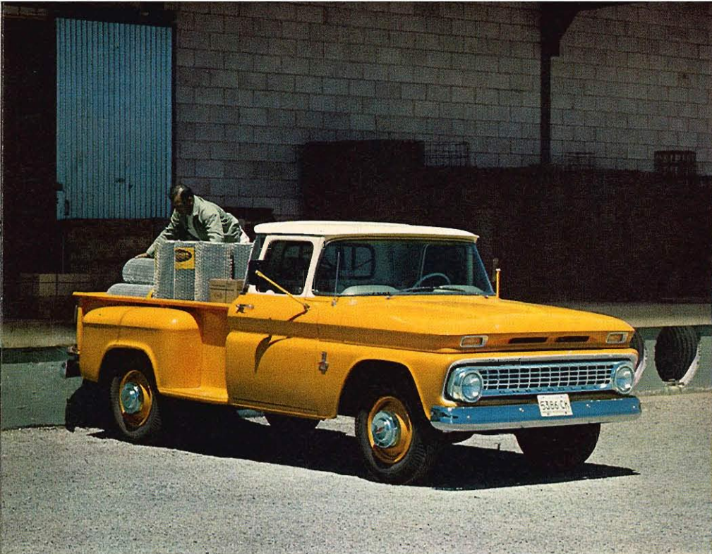
Stepside pickup —Five Stepside models in the ½-, ¾- and one-ton classes with GVW's from 4,100 to 7,800 lbs. are offered with body lengths ranging from 6½ to 9 feet. Durable select wood floors with recessed steel skid strips simplify loading. Wide choice of 6-cylinder or V8 power offers top operating economy for any job.
