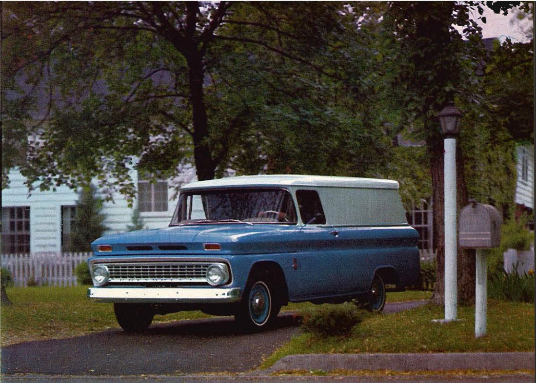
Panel models —Here to handle big loads with ease and efficiency, Chevrolet's 3 new panel models range in GVW's from 4,100 to 7,800 lbs.; carry up to 3,300 lbs. of cargo smoothly with new work-tested independent front suspension with coil springs and new two-stage rear coil springs as standard equipment. Bodies in 7½- and 10½-foot lengths.
