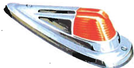
CAB CLEARANCE LAMPS A streamlined lamp that can be installed on any Chevrolet cab or panel body roof.
