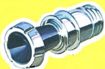
CIGARETTE LIGHTER AND LAMP —Lighter well is lighted when headlamps are turned on for easy replacing of lighter.
