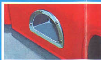
PICK-UP SIDE STEP Permits easy access to the cargo in the front load space of the pick-up box.
