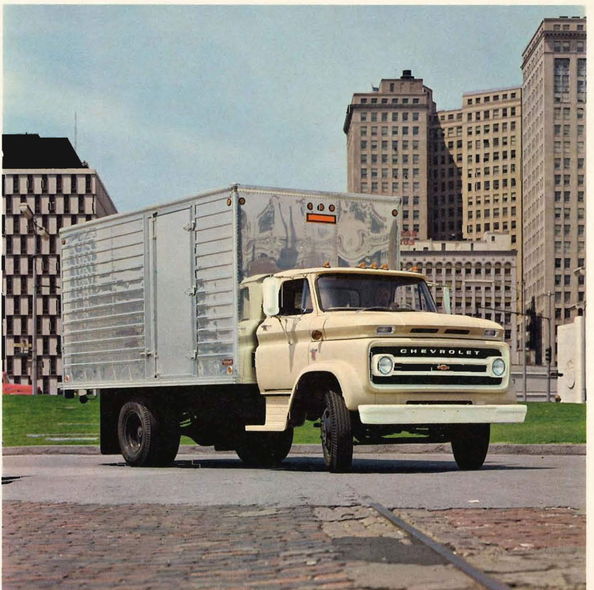
1964 CHEVROLET LOW-CAB-FORWARD MEDIUM-DUTY TRUCKS —Just 93 inches from bumper to back of cab, these space-saving low-cab-forward models are available as both Series 50 or Series 60 models. Engine, frames, suspensions and other components are of the same tough quality as those in their conventional-cab counterparts, but offer the added value of short-wheelbase compactness and maneuverability.
