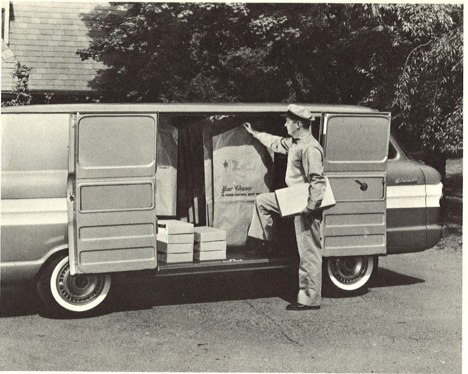
Big right-side double doors open on a spacious curb level load compartment with 4½ feet of head room for easy cargo handling.
