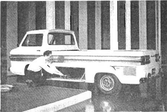
PICKUP IS A TRUE LOADSIDE WITH A FULL LENGTH FLAT FLOOR AND OPTIONAL PANORAMIC REAR WINDOW.
