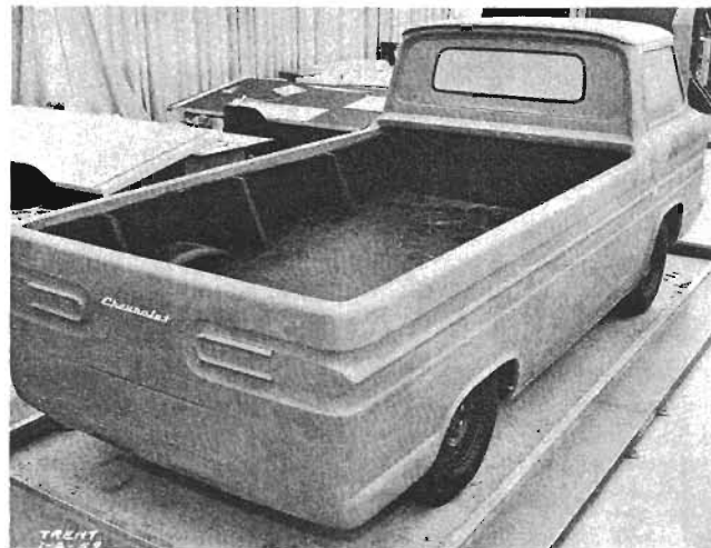
THE LOADSIDE PICKUP TAKING SHAPE IN THE CHEVROLET TRUCK STUDIO AT GM STYLING. (1-2-59)
