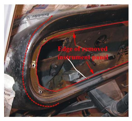
I decided it would be easier to refinish the inside of the old and replacement dashes prior to reinstallation. The <u>fourth</u> <u>figure</u> shows the original dash after the front was removed and the underside was stripped, primed and painted. The weld seam was refinished afterwards.
