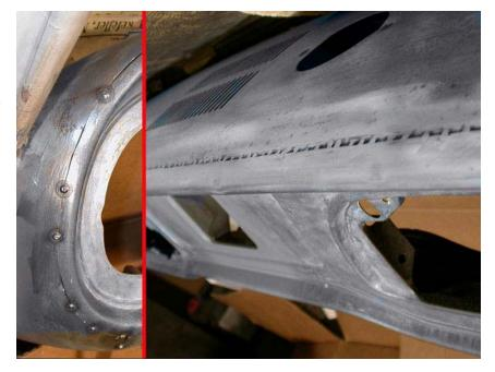
The welds were ground flush, and the seam given a little filler, and sanded smooth (Figure 9 and 10). Because of the location, the seam is almost invisible when viewed from the underside. It was nevertheless primed and painted.
