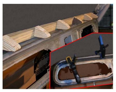
Assorted clamps to the window posts, etc. were used to align the edges (Figure 7). With the accurate cuts, alignment was not difficult to achieve.
