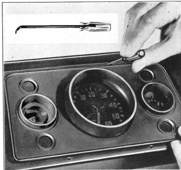
Fig. 2—Instrument Cluster Retaining Clip Depressor
