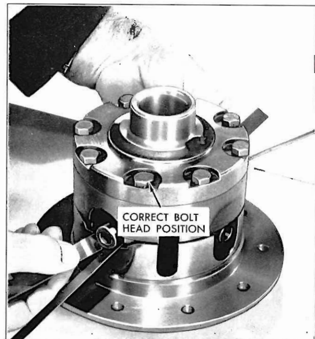
Fig. 1—Checking Mate Shaft Clearance
