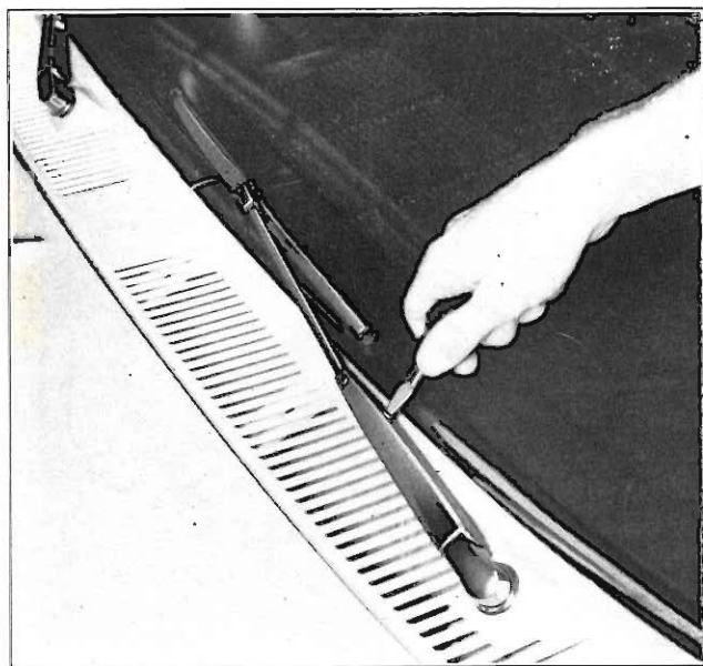
Fig. 8—Adjusting Wiper Blade Park
