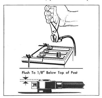
Fig. 1—Installing Spring Ring Clamp
