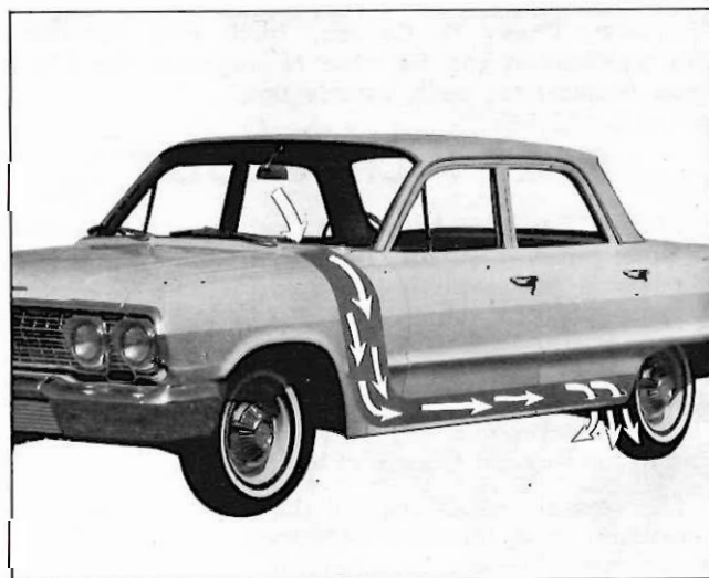
Fig. 2—Rocker Panel Air Flow
