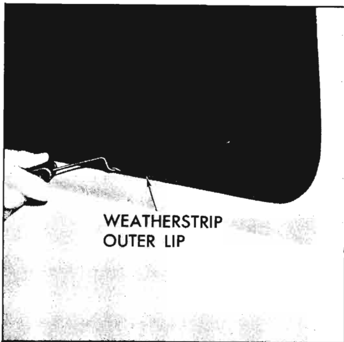
Fig. 10-92a—Installing Rear Quarter Window Weatherstrip
