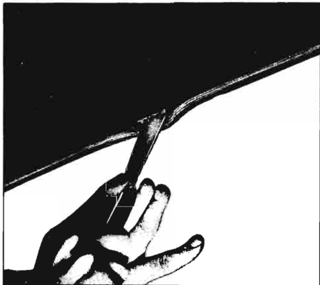
Fig. 10-18a—Loosening Windshield Weatherstrip
