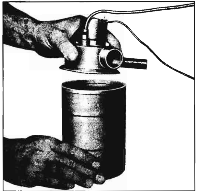
Fig. 11-7—Installing Burner on Checking Gauge J-8367
