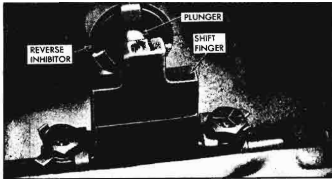
Fig. 6D-48—Reverse Inhibitor and Shift Finger Installation
