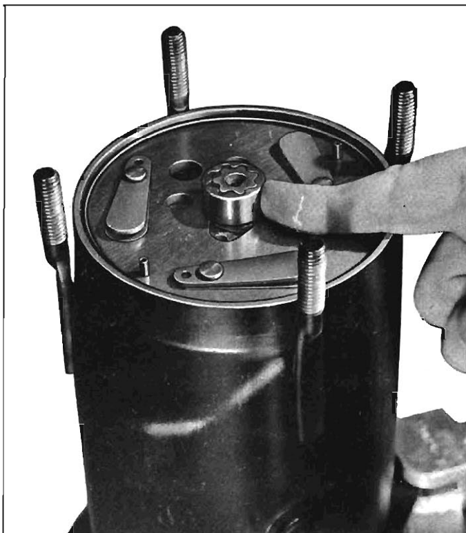
Fig. 11-44—Proper Oil Pump Gear Positioning
