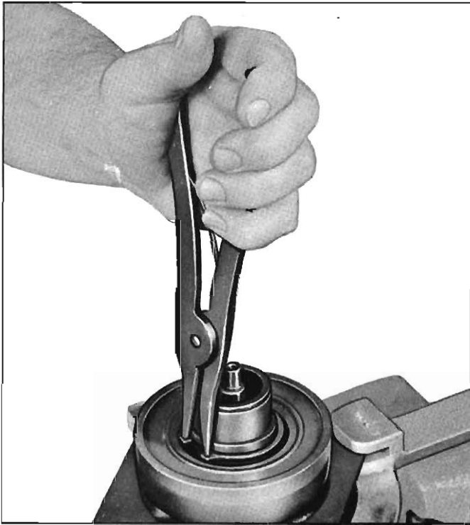
Fig. 11-37—Removing Coil Housing Retainer Ring
