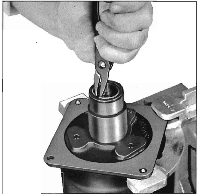
Fig. 11-40—Removing Seal Seat Retaining Snap Ring
