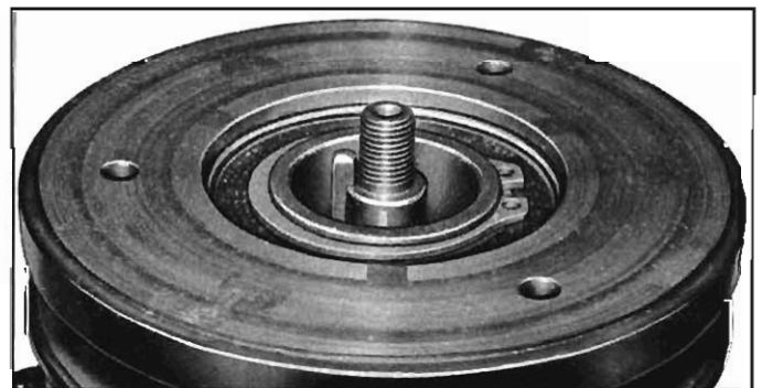
Fig. 11-33—Drive Plate Key Installed in Keyway
