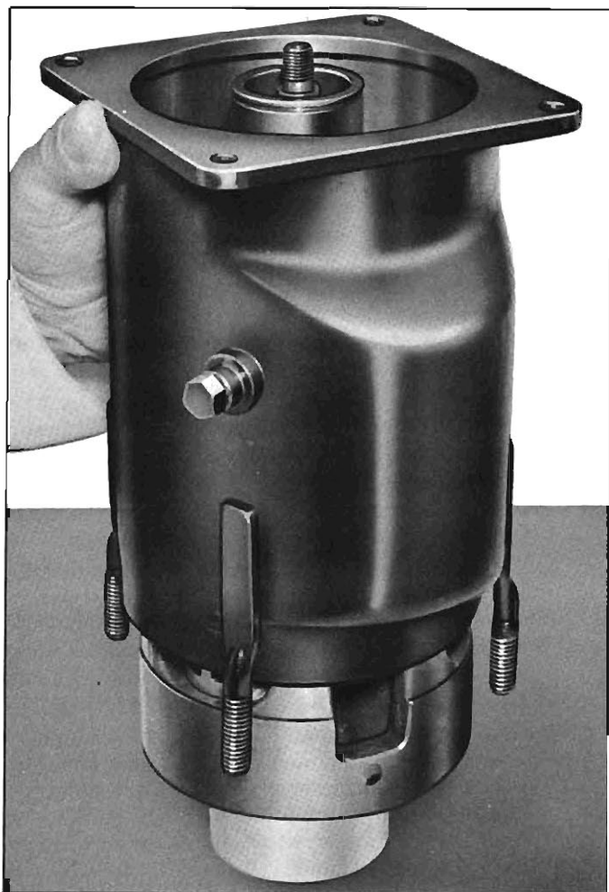
Fig. 11-56—Installing Shell Over Internal Mechanism
