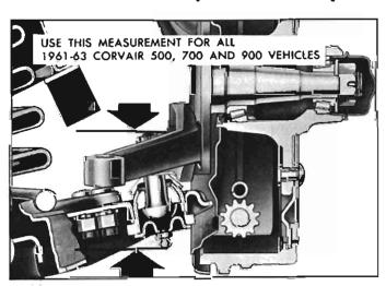
Fig. 3-1—Checking Lower Spherical Joint
