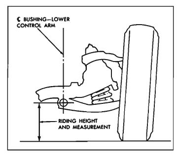
Fig. 3-2-Front Pivot Height
