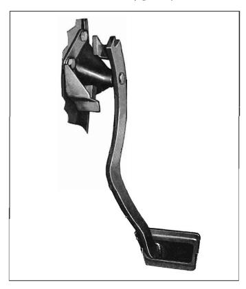
Fig. 68-1—Clutch Linkage
