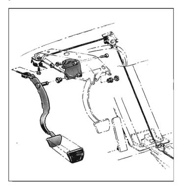
Fig. 6B-2—Pedal Support Bracket
