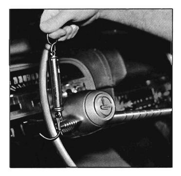
Fig. 1—Checking Steering Adjustment
