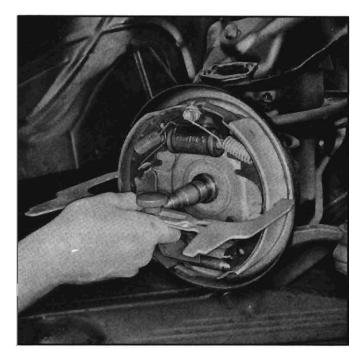
Fig. 5-13—Checking Brake Shoe Lining Clearance
