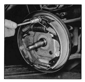
Fig. 5-8—Unhooking Pull Back Springs
