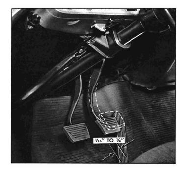
Fig. 5-5-Brake Pedal Free Movement
