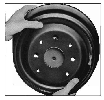
Fig. 5-14—Aligning Drum Tang with Axle Shaft
