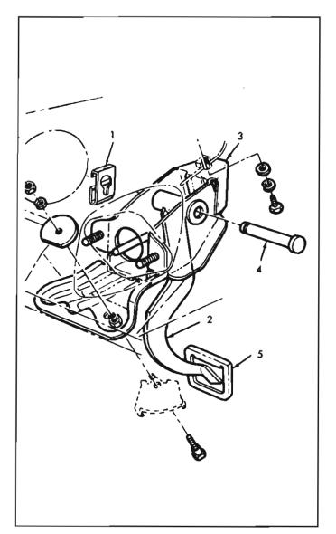
Fig. 5-7-Brake Pedal and Attaching Parts
