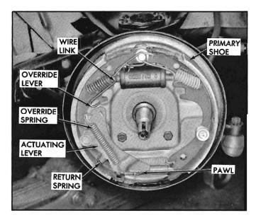
Fig. 5-1-Self-Adjusting Brakes
