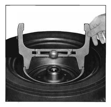
Fig. 5-12-Using Drum-to-Brake Shoe Clearance Gauge
