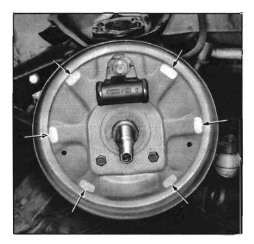
Fig. 5-10-Backing Plate Contact Faces
