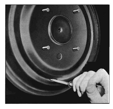
Fig. 5-2-Brake Drum Access Hole
