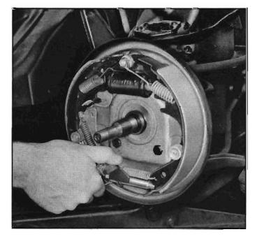
Fig. 5-11—Checking Operation of the Actuating Lever
