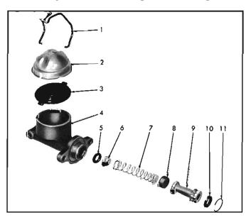
Fig. 5-6-Brake Main Cylinder
