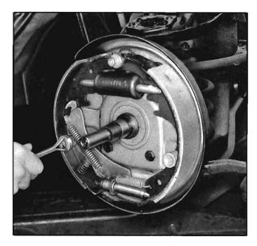
Fig. 5-9—Removing Hold Down Springs and Pins
