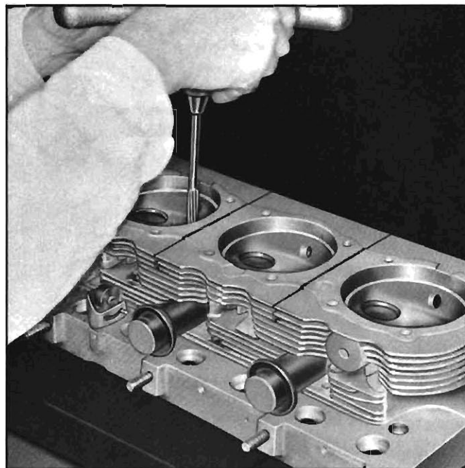
Fig. 10—Reaming Cylinder Head Valve Guide Bore
