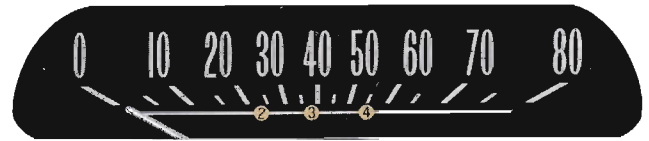
A speedometer indicating maximum upshift speeds is an additional feature on Greenbriers equipped with a 4-speed transmission.
