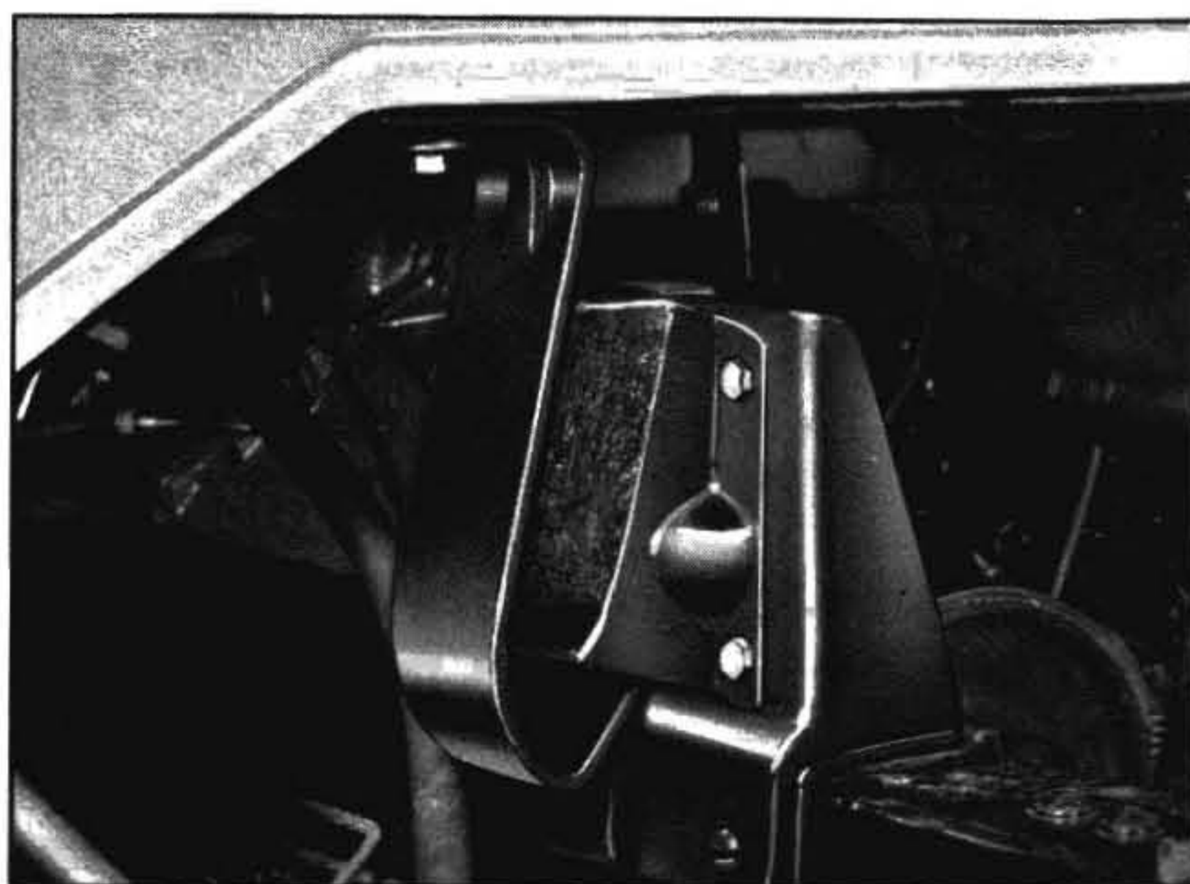
Fig. 4-5—Shear Type Cab Mounts L50 to 80
