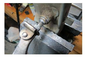
The new spline was clamped in place. Make sure surfaces of the spline and the shaft are nice and flat. It makes clamping much easier.
