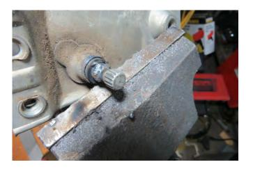
They were then welded together. The weld really didn't need to be cleaned up in this case since the handle slipped on all the way. It's all out of sight when to handle is in place.
