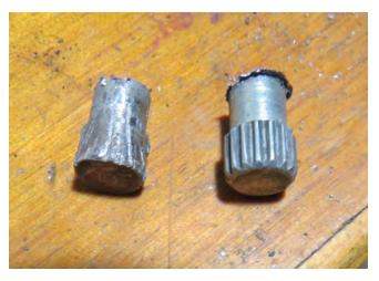
From the step out, the Corvair splines were exactly the same length.
