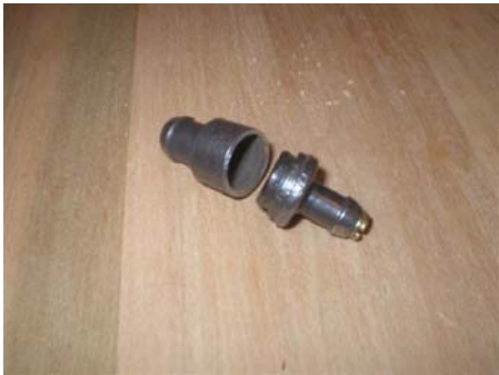
Photo 2 With the inner valve and spring removed, flow brazing rod into the small end. Drill with a no. 3 drill bit and thread with a 1/4"-28 tap and screw in a carb jet. I drilled out mine to .062 which is the size recommended for most 64-69 engines in the service manuals. However, I checked the orifice size on seven engines and the size ranged from .055 to .096. Perhaps GM thought the size was not that critical, or they could have been enlarged from cleaning.
