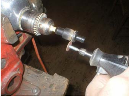
Photo 1 A 5/16" wood dowel rod is inserted into the valve and chucked into a variable speed drill. A Dremel tool with a cut-off wheel is used while the drill is rotating at a slow speed to cut the PCV valve (proper eye protection must be used). Make the cut approximately 3/16" from the raised shoulder on the valve as there is an inner sleeve in this area that aids in brazing the valve back together.
