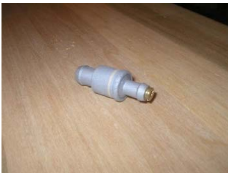
Photo 3 The valve is brazed together, and excess material is filed, sanded, and media blasted. The result is an empty PCV valve with a fixed orifice at one end.
