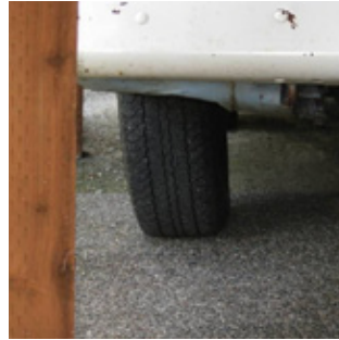
Before the typical FC positive rear camber that eats the outside of the tire.
