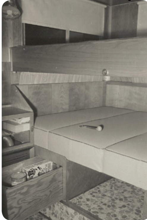
The camper is fitted with bunk beds (left). The top bunk can be cranked up allowing a dinette table to be installed when needed (right).
