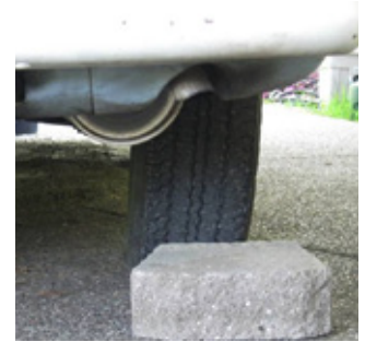
Before the typical FC positive rear camber that eats the outside of the tire.
