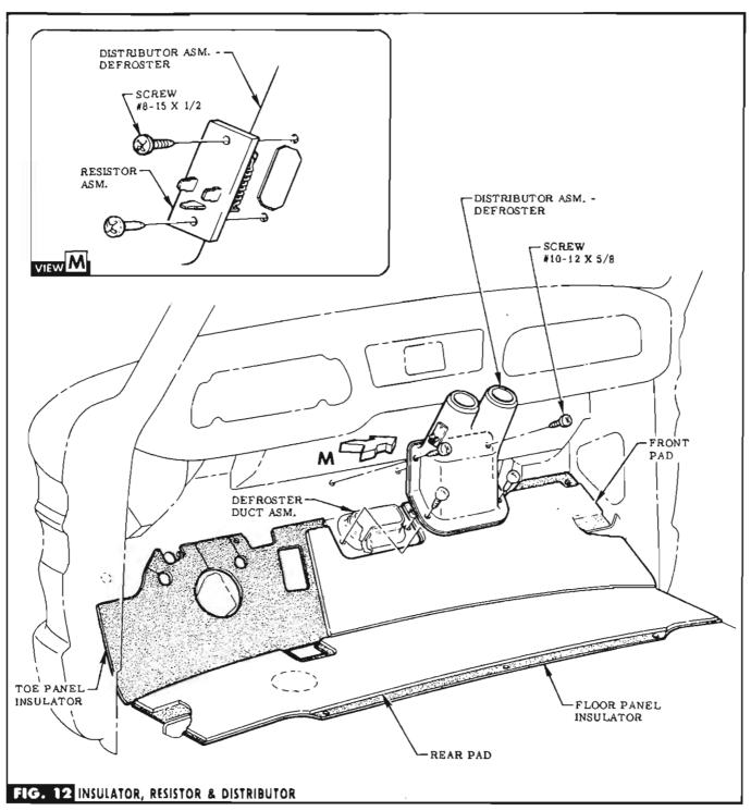
STEP 49 CEMENT TOE PANEL & FLOOR PANEL INSULATORS TO UNDERBODY. SEE FIG. 12.
