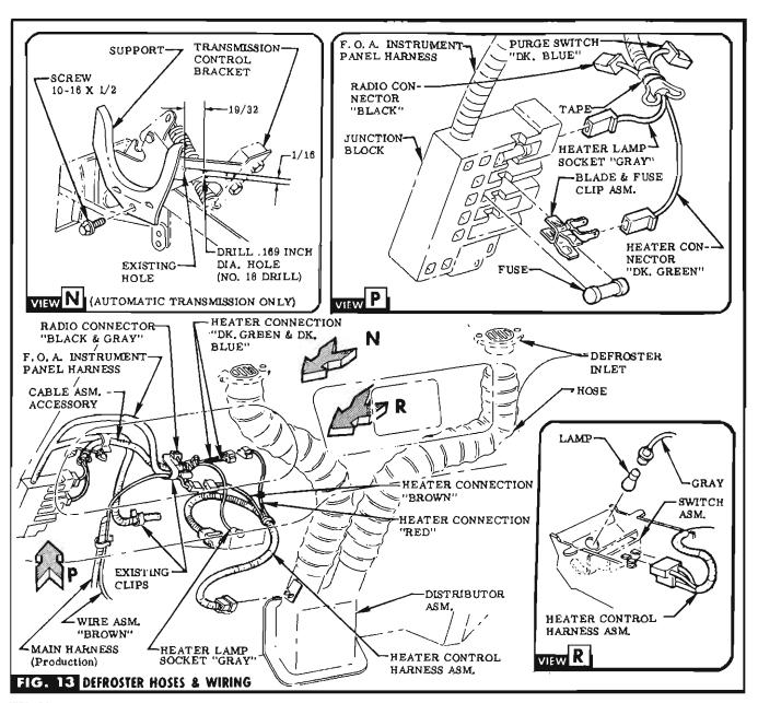
STEP 53 IF AUTOMATIC TRANSMISSION EXISTS, INSTALL HOSE SUPPORT ON TRANSMISSION CONTROL BRACKET WITH SCREW PROVIDED (IN BAG A). SEE VIEW N.
