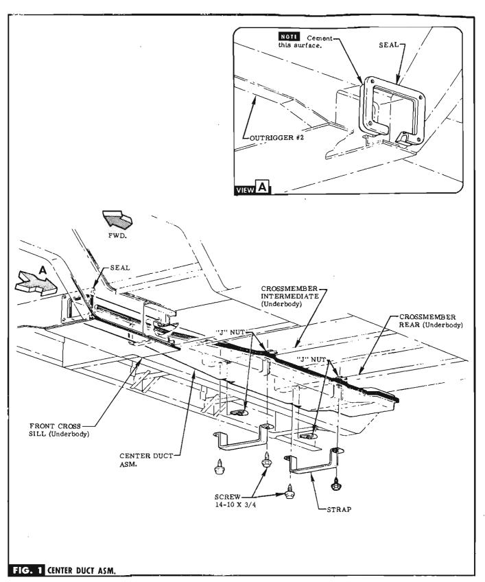
STEP 1 CEMENT SEAL TO OPENING ON REAR SIDE OF OUTRIGGER #2 & SLIP J-NUTS (IN BAG B) INTO PLACE ON INTERMEDIATE & REAR CROSSMEMBER. SEE FIG. 1 & VIEW A.
