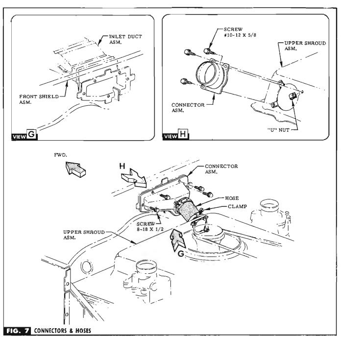
STEP 26 INSERT HAND THRU OPENING & PULL INLET DUCT THRU. INSTALL CONNECTOR WITH SCREWS PROVIDED (IN BAG D). SEE FIG. 7 & VIEW G.
