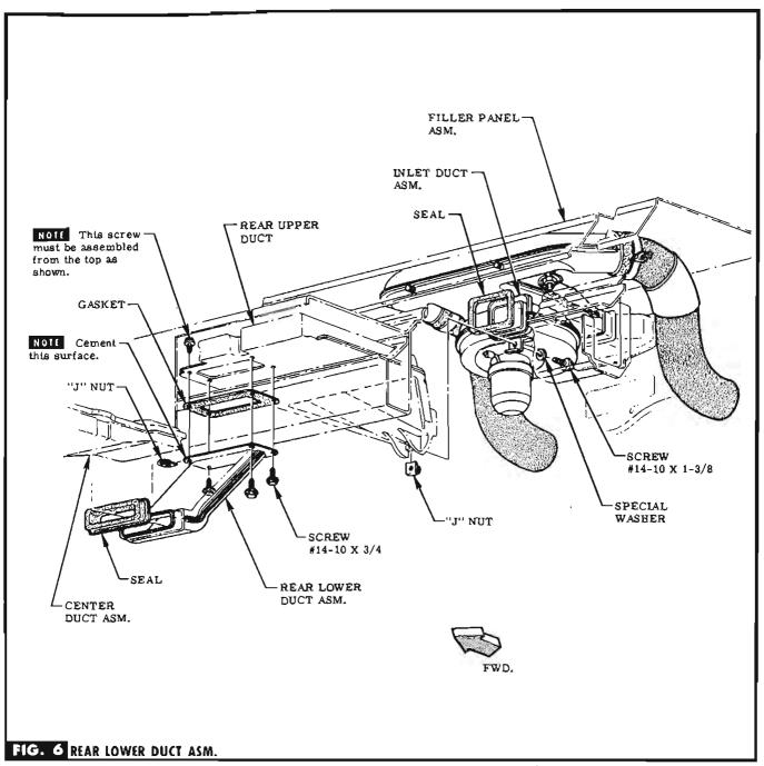
STEP 22 SLIP J-NUT (IN BAG C) INTO PLACE. CEMENT SEAL TO INLET DUCT. SEE FIG. 6.
