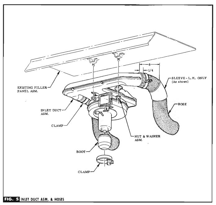
STEP 18 REMOVE FILLER PANEL ASM. & ATTACHING PARTS & RETAIN.
