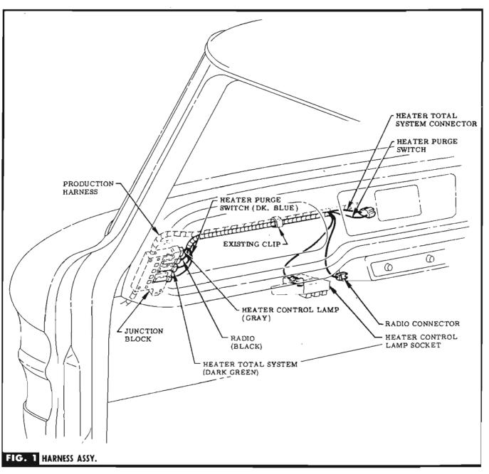
**STEP 1** PLUG LEADS INTO JUNCTION BLOCK ONLY IF CON-CERNED WITH ACCESSORY SPECIFIED. SEE FIG. 1.
