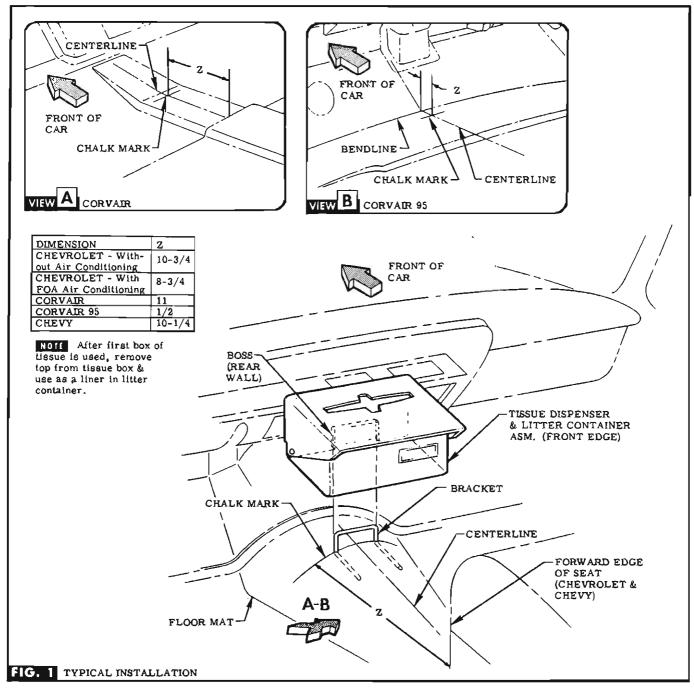
NOIL Be sure floor mat surface is clean & dry for marking dimensions when installing container.
