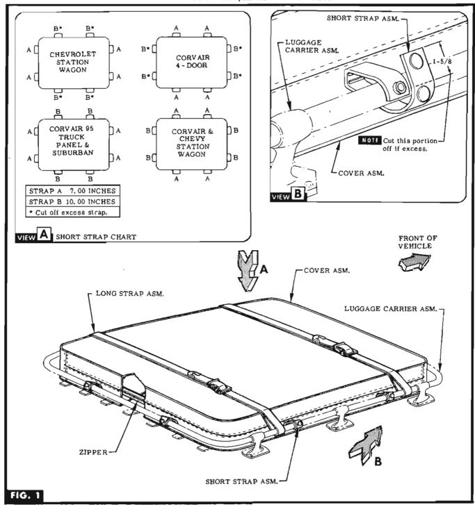
STEP I PLACE COVER ASM. INSIDE ROOF LUGGAGE CARRIER ASM. WITH SHORT STAPLED STRAPS (DOWN) ON LOWER HALF & ZIPPER FACING TOWARD REAR & RIGHT SIDE OF VEHICLE. SEE FIG. 1.
