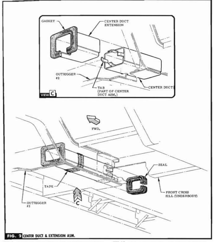
STEP 9 INSTALL GASKET ONTO CENTER DUCT EXTENSION, SEE VIEW C.
