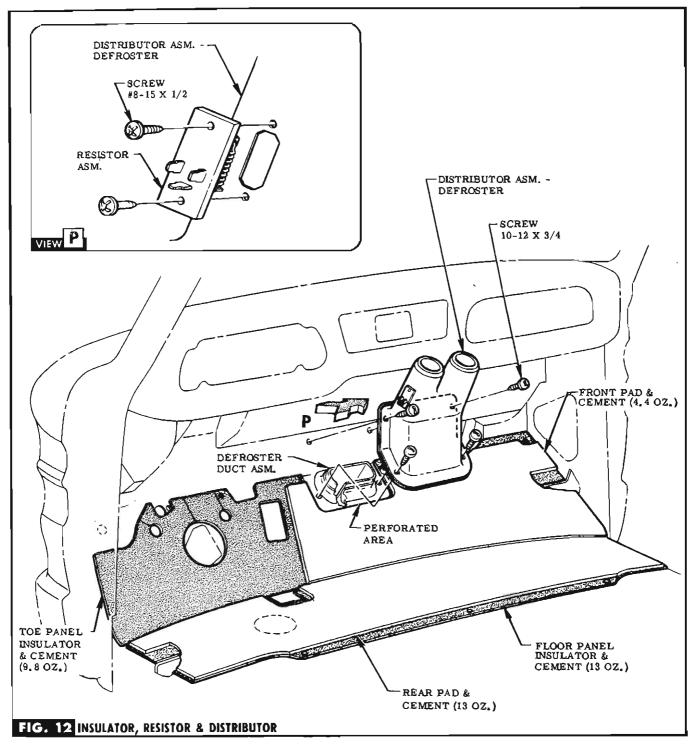
**STEP 58** REMOVE EXISTING FLOOR MAT & CEMENT PRO-VIDED PADS TO UNDERBODY OF FLOOR MAT. CUT OUT PERFORATED AREA. SEE FIG. 1.
