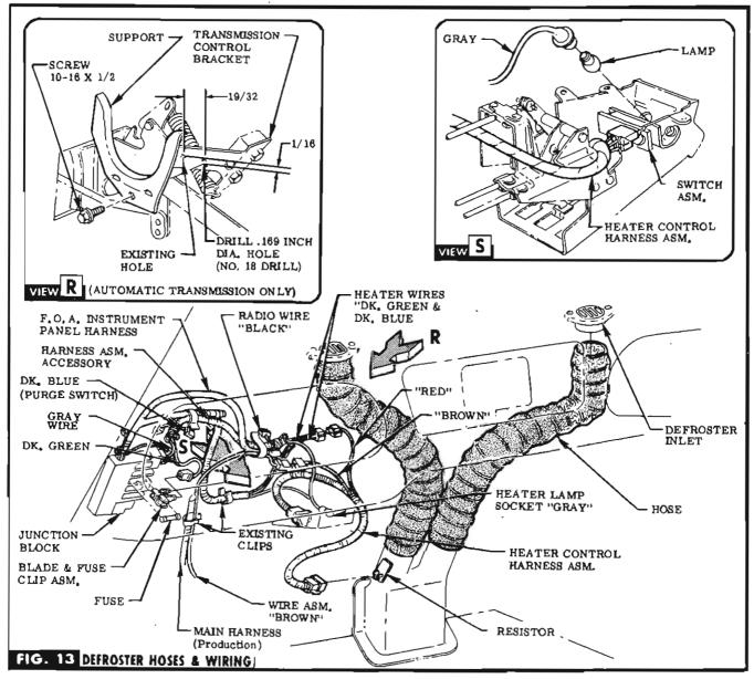
**STEP 62** AUTOMATIC TRANSMISSION EXISTS, INSTALL HOSE SUPPORT ON TRANSMISSION CONTROL BRACKET WITH SCREW PROVIDED (IN BAG A). SEE VIEW R.
