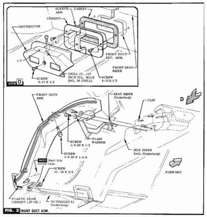
**STEP 15** CEMENT GASKET TO SLEEVE & SLIDE SLEEVE THRU OPENING IN SEAT RISER & INTO FRONT DUCT EX-TENSION. ATTACH WITH SCREWS (IN BAG A). SEE VIEW D.
