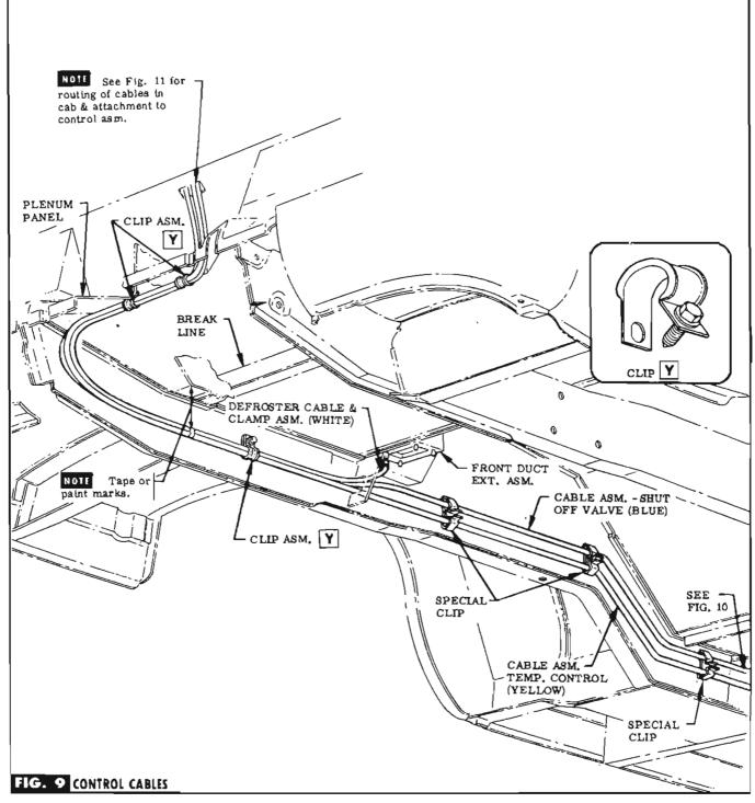
**STEP 46** ALIGN TAPE OR PAINT MARKS ON THE CABLES DIRECTLY BELOW FLOOR TO TOE PANEL BREAK LINE BE-FORE CLIPPING TO UNDERBODY. ROUTE CABLES ALONG. RIGHT SIDE RAIL & ATTACH TO EXISTING HOLES IN PLENUM PANEL & SIDE RAIL WITH CLIPS (IN BAG B). SEE FIG. 9.
