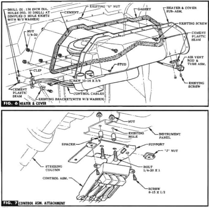
STEP 28 REMOVE EXISTING R. H. AIR VENT ROD & TUBE ASM. & DISCARD, RETAIN ATTACHING PARTS.
