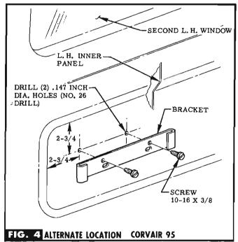
USING BRACKET AS A TEMPLATE, CENTER PUNCH & DRILL HOLES. SEE FIG. 3.
