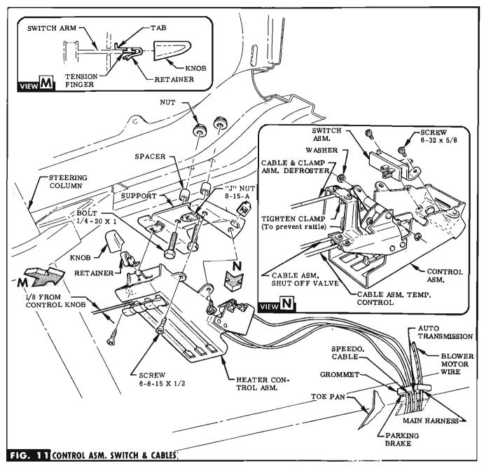
**STEP 51** REMOVE GROMMET RETAINER FROM TOE PANEL & DISCARD EXISTING GROMMET. ROUTE CONTROL CABLES & BLOWER MOTOR WIRE THRU OPENING IN TOE PANEL & THRU GROMMET (IN BAG A). POSITION GROMMET & THEN SECURE WITH EXISTING RETAINER. SEE FIG. 11.
