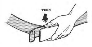
TO LOOSEN BELT TURN BUCKLE OUTWARD
