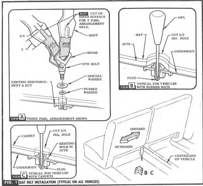
STEP I USING DIMENSIONS GIVEN, LOCATE PLUG BY FEEL-ING CARPET (SLIGHT INDENTATION) OR UNDER RUBBER MAT (SLIGHT HUMP). PROBE WITH AWL TO LOCATE HOLE IN PLUG. INSERT AWL DOWN INTO PLUG & LEAVE STANDING IN UPRIGHT POSITION, CUT CARPET OR MAT. SEE FIG. 1 (VIEW B & C) & FIG. 2 - CHEVROLET
