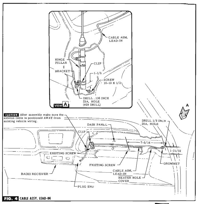
STEP 9 WITH CLIP LOCATED TO DIMENSION SHOWN & ANTENNA ASM. IN VERTICAL POSITION, USE BRACKET AS A TEMPLATE & DRILL A HOLE IN HINGE PILLAR. SEE VIEW A.
