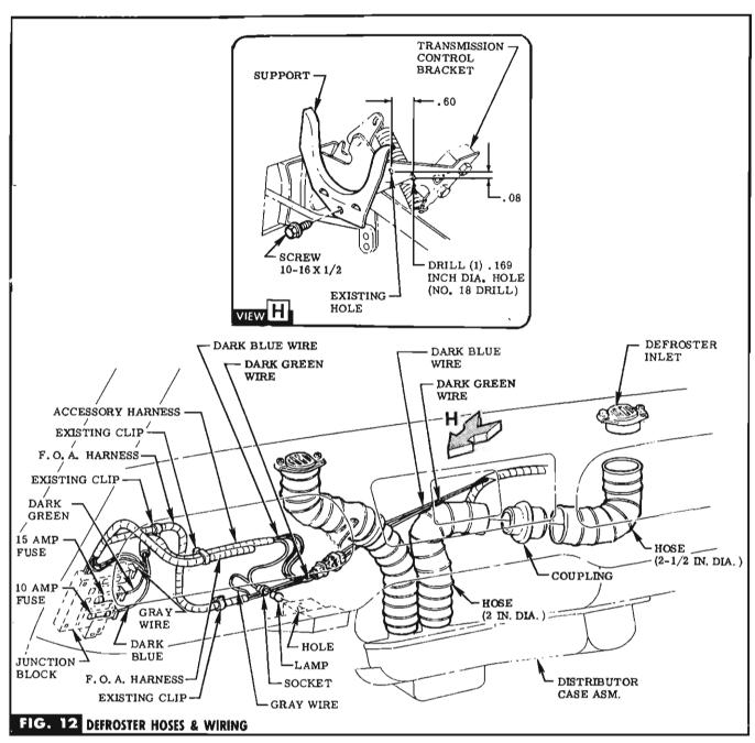
**STEP 58** IF AUTOMATIC TRANSMISSION EXISTS, DRILL HOLE & INSTALL HOSE SUPPORT ON TRANSMISSION CONTROL BRACKET WITH SCREW (IN BAG A). SEE VIEW. H.
