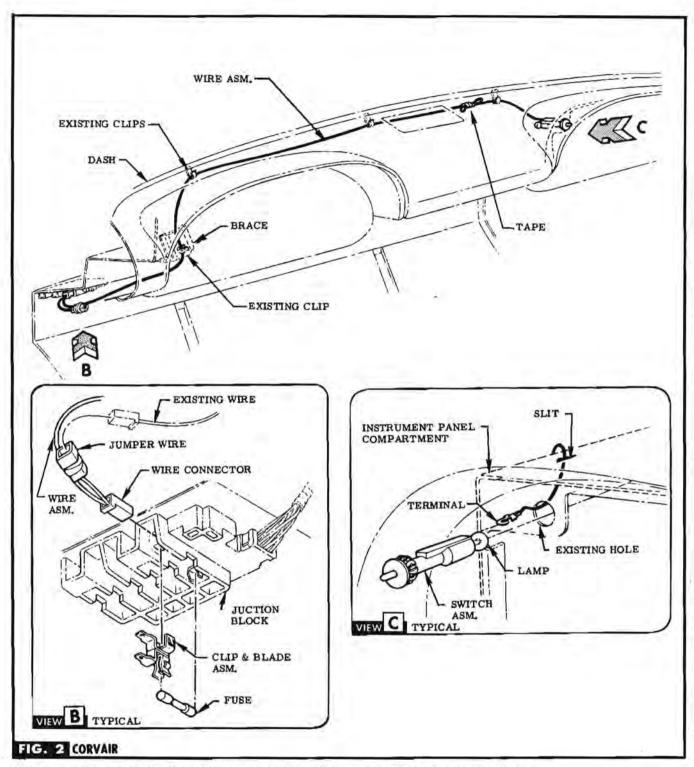
STEP 10 ROUTE WIRE TERMINAL THRU SLIT IN UPPER LEFT HAND CORNER OF INSTRUMENT PANEL COMPARTMENT & THRU HOLE IN UPPER LEFT SIDE OF COMPARTMENT OPENING. SEE FIG. 2 & VIEW C.
