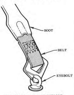
BELT ATTACHMENT TO EYEBOLT (WITH BOOT IN RAISED POSITION)
