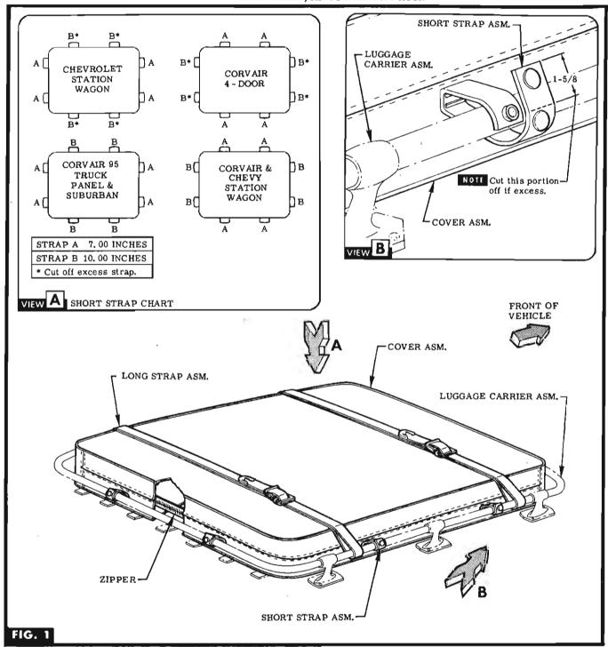
**STEP 1** PLACE COVER ASM. INSIDE ROOF LUGGAGE CARRIER ASM. WITH SHORT STAPLED STRAPS (DOWN) ON LOWER HALF & ZIPPER FACING TOWARD REAR & RIGHT SIDE OF VEHICLE. SEE FIG. 1.
