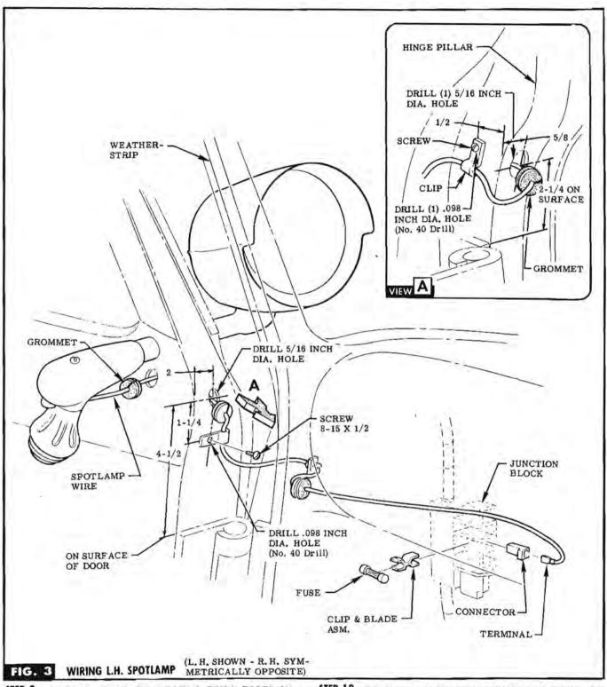
STEP 9 LOCATE, CENTER PUNCH & DRILL HOLES ON FORWARD EDGE OF DOOR & FRONT BODY HINGE PILLAR. SEE FIG. 3 & VIEW A.
