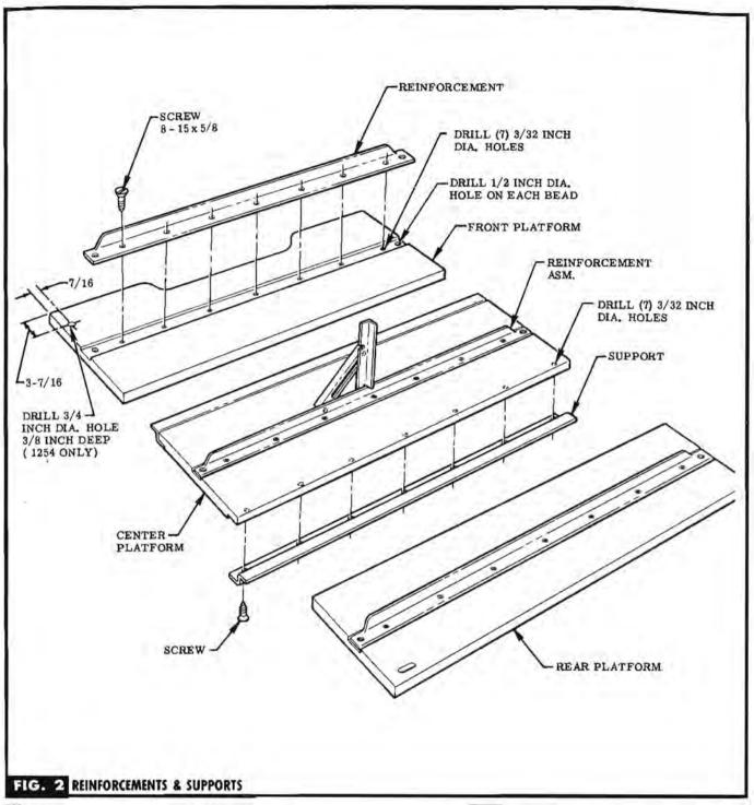
STEP 7 USING REINFORCEMENTS PROVIDED AS A TEM-PLATE, LOCATE & DRILL HOLES IN UNDERSIDE OF PLAT-FORMS. NOTE Do not drill thru plywood with 3/32 inch drill. SEE FIG. 2.
