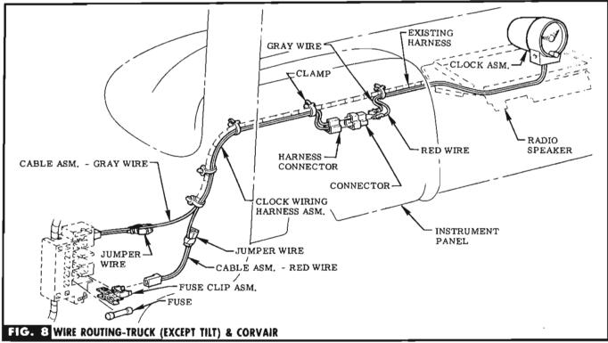
STEP 7 (ALL EXCEPT CHEVY) INSTALL FUSE CLIP & FUSE INTO RECEPTACLE IN JUNCTION BLOCK MARKED "GL. BOX LP." & PLUG IN RED WIRE CONNECTOR. SEE FIG. 5, 6 OR 8. NOTE If receptacle is occupied, remove existing wire & plug into jumper wire. Discard fuse & clip.
