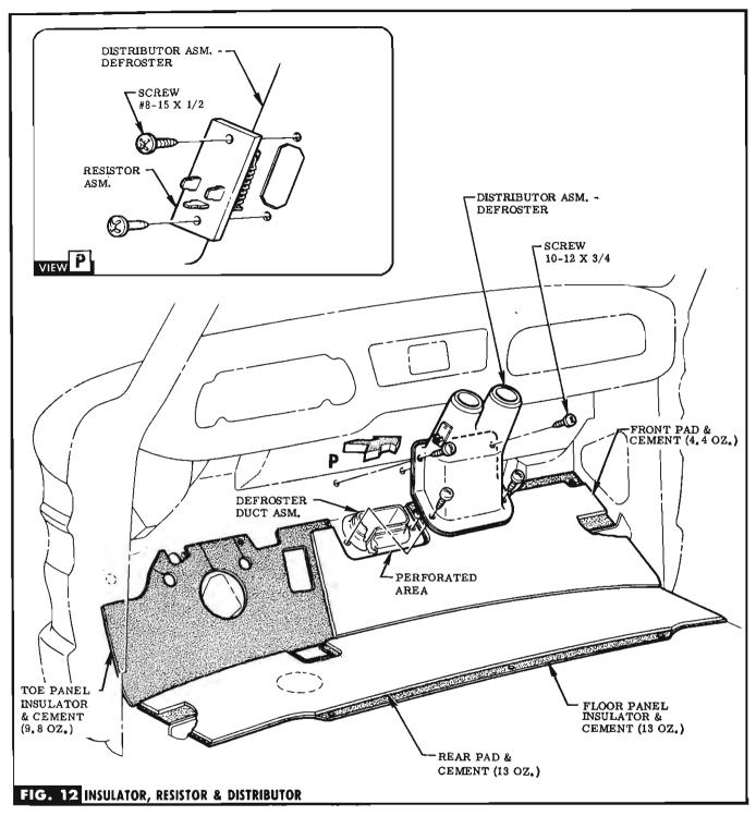
**STEP 58** REMOVE EXISTING FLOOR MAT & CEMENT PROVIDED PADS TO UNDERBODY OF FLOOR MAT. CUT OUT PERFORATED AREA. SEE FIG. 1.
