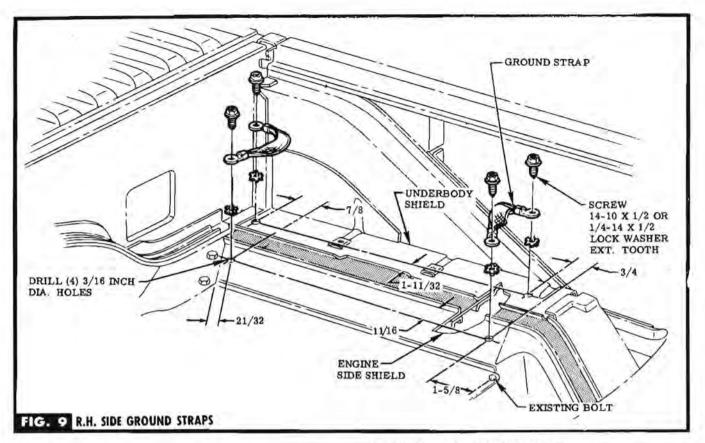
STEP 16 LOCATE, CENTER PUNCH, & DRILL HOLES IN ENGINE SIDE SHIELDS & ENGINE COMPARTMENT UNDERBODY SHIELDS. SEE FIG. 9.
