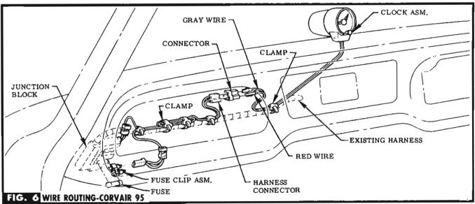
STEP 5 INSERT CABLE INTO 2-WAY CONNECTOR & PLUG IN CLOCK WIRES, MATCHING COLORS. SEE FIG. 5, 6, 7 OR 8.
