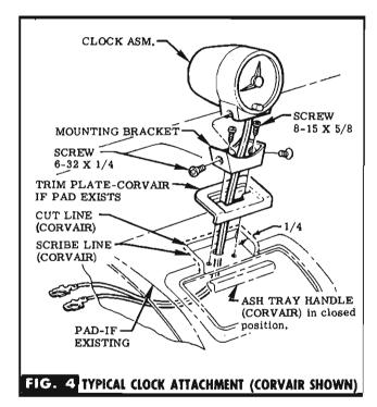
STEP 3 INSERT CLOCK WIRES THRU CENTER HOLE IN MOUNTING BRACKET & TRIM PLATE (IF REQUIRED) & ATTACH BRACKET TO INSTRUMENT PANEL WITH SCREWS, SEE FIG. 4.
