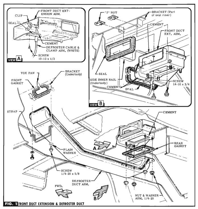
**STEP 1** REMOVE COVER & SCREWS FROM FRONT SEAT RISER & DISCARD.
