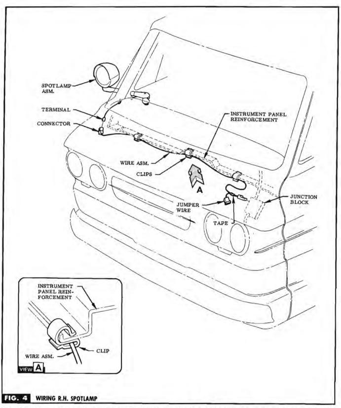
STEP 15 (R.H. SPOTLAMP) PLUG TERMINAL INTO CONNECTOR ON WIRE ASM, INSTALL CLIPS ON INSTRUMENT PANEL REINFORCEMENT AT CONVENIENT LOCATIONS. ROUTE WIRE ASM, THRU CLIPS. SEE FIG. 4 & VIEW A.
