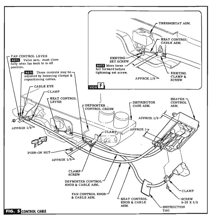
**STEP 23** INSERT FAN, DEFROSTER & HEAT CONTROL KNOB & CABLE ASSEMBLIES INTO SLOTS OF HEATER CONTROL. SLIDE CABLE SHEATHS UP INTO SLOTS & SECURE TO DIMENSION SHOWN WITH CLAMPS & SCREWS (IN BAG A). SEE FIG. 5.
