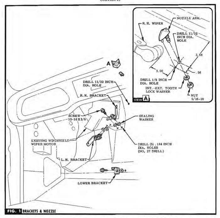
STEP 1 LOCATE EXISTING DIMPLES IN DASH PANEL & DRILL HOLES FOR UPPER R, H, & L, H, & LOWER BRACKETS & GROMMET, SEE FIG. 1. NOTE If heater exists, use lower hole of heater control cables clip for attaching lower bracket.
