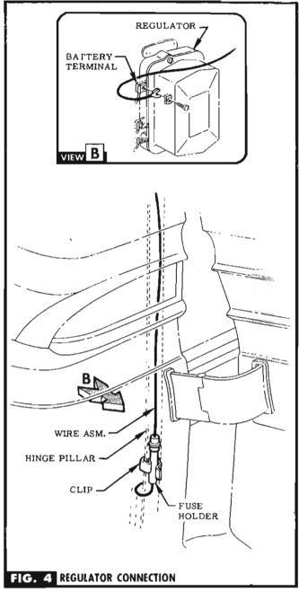
assist routing thru holes & around corners.
