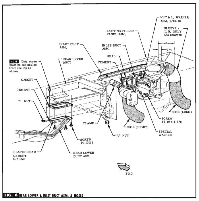
**STEP 28** REMOVE FILLER PANEL ASM. & ATTACHING PARTS & RETAIN.
