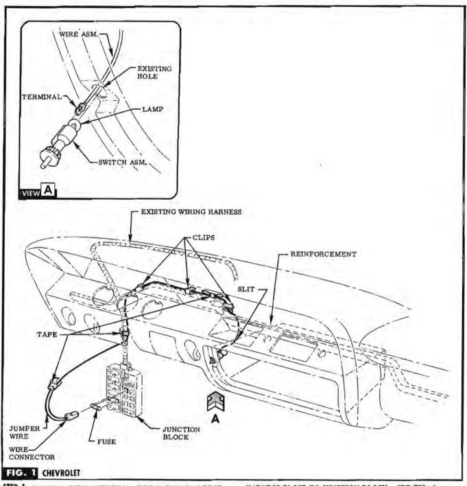
STEP 1 ROUTE WIRE TERMINAL THRU SLIT IN UPPER LEFT HAND CORNER OF INSTRUMENT PANEL COMPART-MENT & THRU HOLE IN UPPER LEFT SIDE OF COMPART-MENT OPENING, SEE FIG. 1 & VIEW A.
