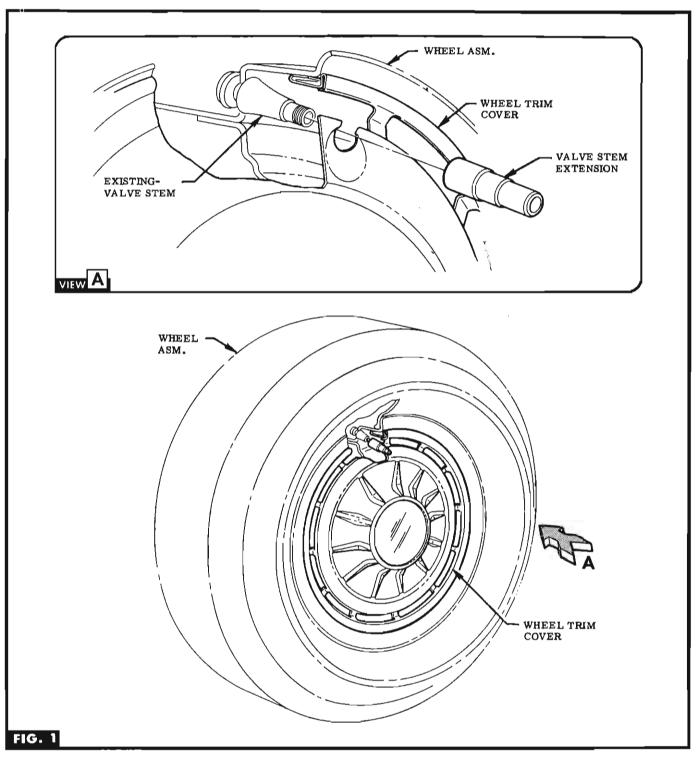
**STEP 1** ATTACH VALVE STEM EXTENSION TO EXISTING VALVE STEM OF EACH WHEEL. SEE VIEW A.
