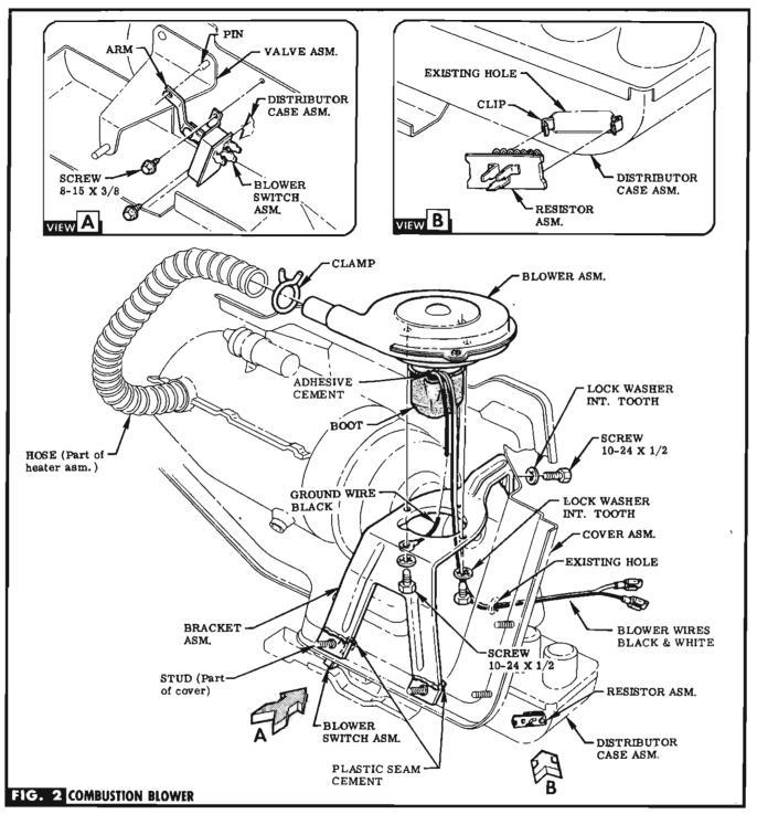
**STEP 6** PLACE BLOWER SWITCH ARM ON VALVE PIN & ATTACH TO DISTRIBUTOR CASE WITH ATTACHING SCREWS PROVIDED (IN BAG A). SEE VIEW A.
