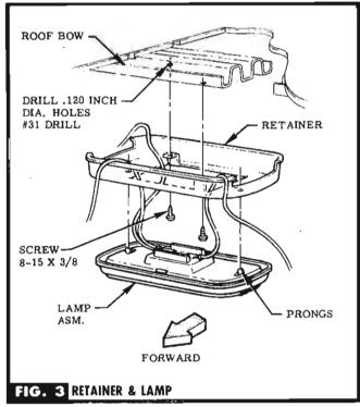
STEP 7 POSITION RETAINER ON CENTER OF REAR ROOF BOW & USE IT AS A TEMPLATE TO DRILL HOLES. SEE FIG. 3. CAUTION Do not drill thru roof panel.
