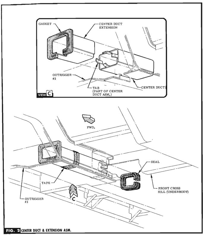
STEP 9 INSTALL GASKET ONTO CENTER DUCT EXTENSION. SEE VIEW  $\text{C}_{\:\raisebox{1pt}{\text{\circle*{1.5}}}}$
