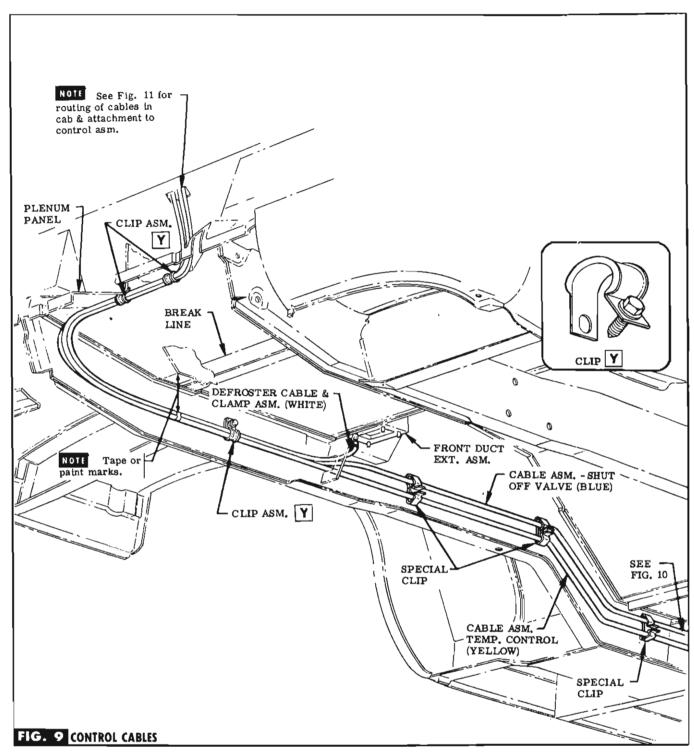
STEP 46 ALIGN TAPE OR PAINT MARKS ON THE CABLES DIRECTLY BELOW FLOOR TO TOE PANEL BREAK LINE BEFORE CLIPPING TO UNDERBODY. ROUTE CABLES ALONG. RIGHT SIDE RAIL & ATTACH TO EXISTING HOLES IN PLENUM PANEL & SIDE RAIL WITH CLIPS (IN BAG B). SEE FIG. 9.
