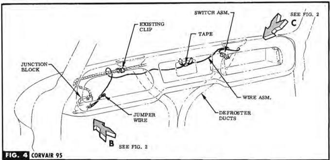
STEP 1b ROUTE WIRE TERMINAL THRU SLIT IN UPPER LEFT HAND CORNER OF INSTRUMENT PANEL COMPART-MENT & THRU HOLE IN UPPER LEFT SIDE OF COMPART-MENT OPENING. SEE FIG. 3 OR 4 & VIEW C, FIG. 2.
