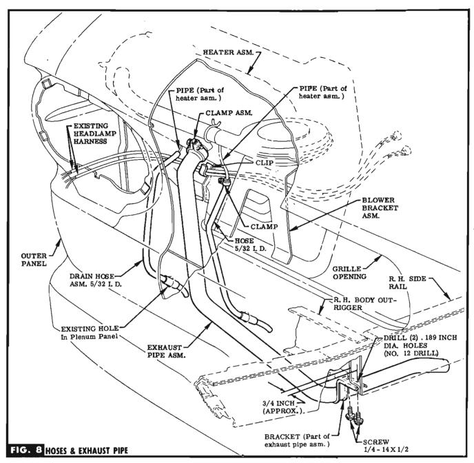
STEP 36 INSERT EXHAUST PIPE THRU EXISTING OPENING IN PLENUM PANEL, FIT CLAMP ASM, PROVIDED OVER TOP & SLIDE EXHAUST PIPE OVER HEATER PIPE. SEE FIG. 8.
