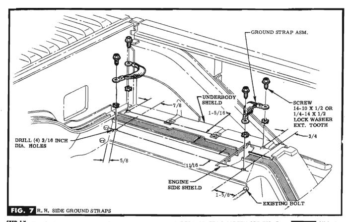
STEP 17 LOCATE, CENTER PUNCH, & DRILL HOLES IN ENGINE SIDE SHIELDS & ENGINE COMPARTMENT UNDERBODY SHIELDS. SEE FIG. 7
