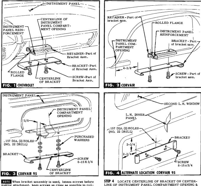
making attachment, keep screws as close as possible to rolled flange.
