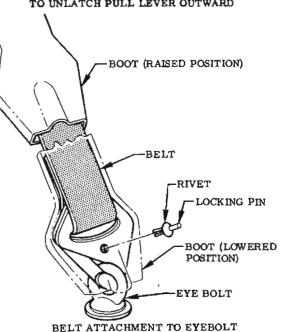
(WITH RIVET IN REMOVED POSITION)
