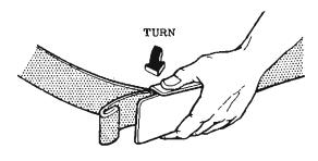
TO LOOSEN BELT TURN BUCKLE OUTWARD
