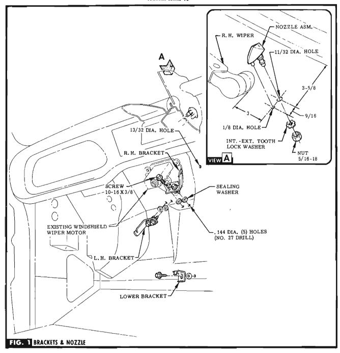
STEP 1 LOCATE EXISTING DIMPLES IN DASH PANEL & DRILL HOLES FOR UPPER R. H. & L. H. & LOWER BRACKETS & GROMMET. SEE FIG. 1. NOTE If heater exists, use lower hole of heater control cables clip for attaching lower bracket.
